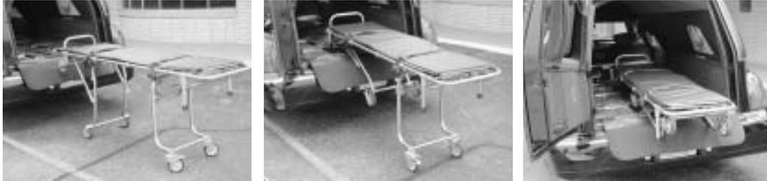
To remove the Mortuary cot from the vehicle, pull cot out of vehicle approximately half-way and pull the red handle. The first set of wheels drop and extend again. Release red handle and pull rest of the way out of the vehicle. The second set of wheels will drop and you should feel them snap into position.
